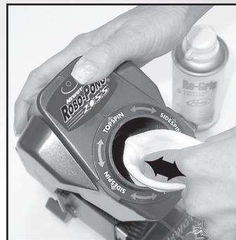
Using a dry, clean section of the cloth, wipe the Friction Block lightly to remove any remaining cleaner and dirt and dry the wheel off.
